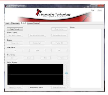
Click 'Begin Testing', this will initiate a scan of the unit to detect the appropriate settings. Once the unit type has been detected the buttons will be populated, click on the appropriate mechanism which needs to be tested.
