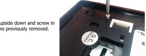
Turn the unit upside down and screw in the 2xT8 screws previously removed.
