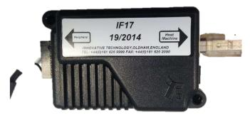
If the unit is connected, enter device manager and check the active com ports, there should be a device labelled as USB Serial. If no com port is present replace the IF17 and a new device will register.
