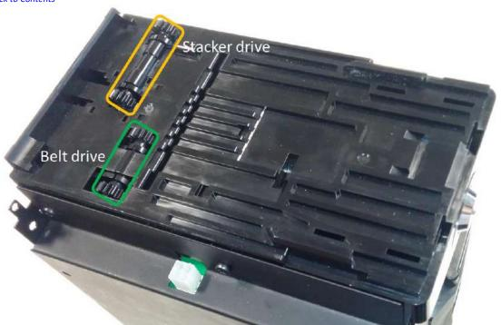
Once the debris has been cleared check foam strips on the stacker to ensure they are not damaged, if not move the stacker back into the rest position. If they are damaged, remove the stacker plate by pushing up and replace the strips with ITL part number LB2034.
