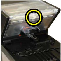
Normal tape position – diverter in CLOSED
