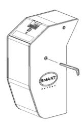
4. Transfer all the stored bank notes onto the Transaction Drum by turning the Allen key clockwise. The barcode will be travelling towards the note exit and the bank notes will be travelling into the module.
