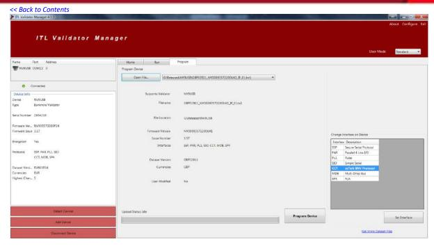
Recently the processor has been changed leading to 2 different versions of firmware being available. If the wrong file for this validator is selected the 'Program Device' button will be greyed out. Details of the change can be found in <a href="Appendix 10.10">Appendix 10.10</a>.
