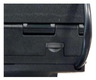
Pressing and holding this button will lead to a test ticket being printed, this ticket will show information on Firmware and the current printer settings.
