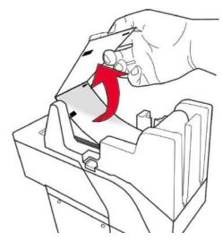
When the paper is inserted into the printer, the TABS need to face towards the NV200.
