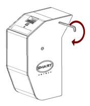
6. Pay out the stored bank notes by turning the Allen key anti-clockwise. The barcode will be travelling into the Payout module and the bank notes will be paid out through the note exit.
