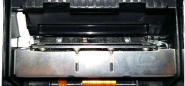
Both the Printer body and the platen (the removed part) can be wiped off with a dampened (NOT wet) soft lint free cloth.
