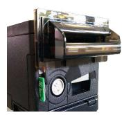
A full guide of how to create an update card can be found in the software manual (GA02037), a link to which can be found in Section 1.1. Once the appropriate card has been generated insert it into the card slot on the NV200. The bezel will begin to flash blue and pink, once the download is complete the bezel will go solid green. Remove the SD card, the NV200 will begin to update any attached device (Payout, Ticket and/or TEBS).
