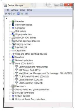
Check the connection to the host software, if there is still an issue replace the IF17 or switch com ports on the PC. If the unit is detected but there is a yellow triangle next to the serial port then the drivers should be reinstalled as explained in <u>Section 6.2.1</u>.
