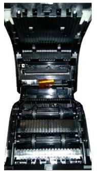
Part of the SMART Ticket needs to be removed so the whole path can be cleaned.
