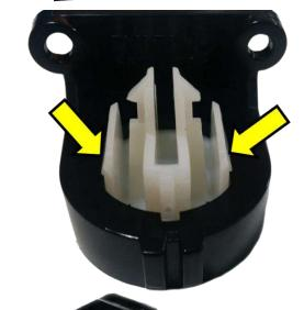
Re-attach the locking cam onto the barrel of the lock and tighten.
