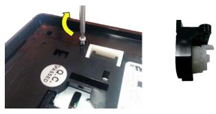
Press the plastic clip together and remove the locking cam.
