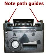
The note path is visible and can be cleaned. Carefully wipe the surfaces with a soft lint free cloth that has been dampened (NOT wet) with a water and mild detergent solution (e.g. household washing up liquid) - be very careful when cleaning around the sensor lenses and make sure they are clean and dry before closing the cover and powering the unit.
