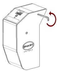
3. Locate the Allen key into the hexagonal Motor Drum slot.
