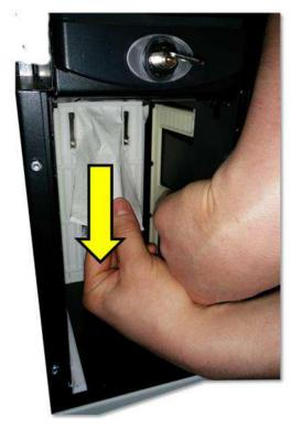
If the note is behind the stacker plate, it is still possible to recover the unit. Wind the stacker plate forward using the gears on top of the TEBS unit as highlighted below. Hold the gear in position while removing the note.
