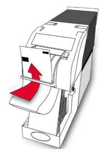
Before being inserted into the printer with the TABS facing towards the NV200.
