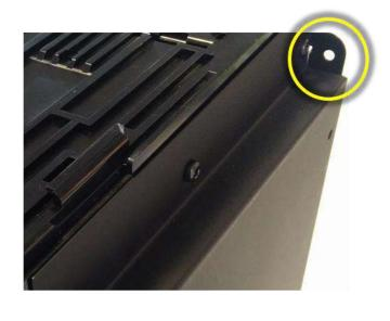
Lack of proper bonding can cause communication issues and other failures. The resistance between the chassis and Earth should be less than  $0.7\Omega$ .
