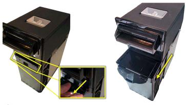
When the cashbox has been removed to access the money, turn it upside down and open the flap as shown in the picture to the right.
