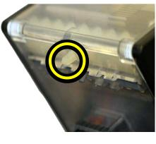
Normal tape position – diverter in OPEN position
