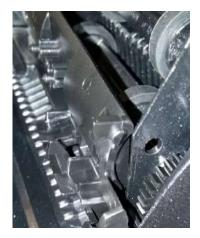
There are Lugs on both sides, when one is unclipped, the other can be removed.
