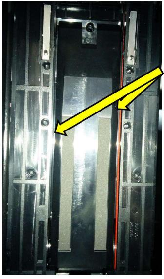
Run cloth down the TEBS belts, ensure you rotate the belt drive so that all of the surface has been cleaned.
