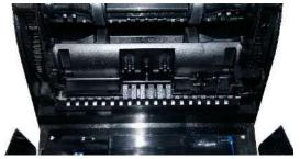
Remove this part by pressing into a lug on the side with a tool (e.g. a screwdriver) and lifting the PM01018 out of position.
