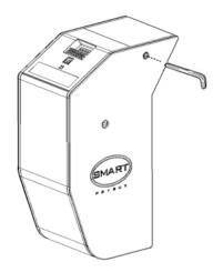
2. Move the Diverter into the transfer position by gently turning the Allen key anti-clockwise until it reaches the dead stop.
