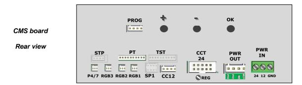
Get access to the menu by holding the three buttons pressed at the same time for 5 seconds.
