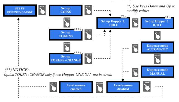
**NOTICE:** monitoring of level sensors is disabled by default. This means that the board does not know when the hopper is empty, so it will send the pay-out command even if there are no coins available. When the hopper runs out of coins during dispensing or at the end of payment, no warning will be displayed. If the empty state is detected when powering the unit, this one shall not accept any money.
