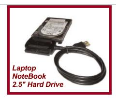
The 2.5" IDE Drive has one connector on the rear. This 44 pin connector is IDE DATA and IDE Power combined. This connector has a blocked socket and must be installed in the correct orientation. Match the blocked socket with the missing pin on the drive mechanism.
